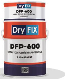
DryFix DFP-600 is a two-component, anticorrosive, zinc phosphate-containing surface-tolerant epoxy primer cured with polyamide hardener. It is used as a surface-tolerant epoxy primer on metal surfaces where sanding or sanding cannot be done, where thin rust cannot be removed, and where only mechanical cleaning can be done. It is suitable for use on working decks, hatch covers, piers and bridge legs, and industrial facility steels.
