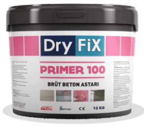
DryFiX PRIMER 100 Exposed concrete primer; is a polymer dispersion based, special mineral added exposed concrete primer. It should be diluted with a maximum of 30% water. It should be stirred frequently during use, the sand should be prevented from settling at the bottom and it should be applied by ensuring that the sand is evenly distributed on the surface.
