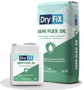
DryFiX SEMI FLEX 2K is a cement-based, polymer-modified, two-component, ready-to-use insulation mortar. It is a two-component, semi-elastic insulation material consisting of a powder component (A component) and a polymer emulsion-based (B component) liquid component, applied before ceramic flooring to provide waterproofing.
