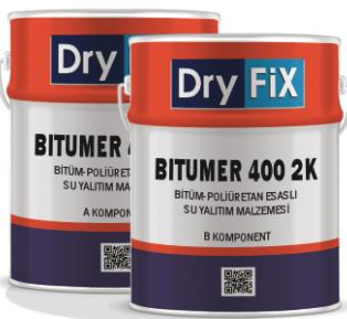
DryFix BITUMER 400 2K is a fast curing, two-component, bitumen-enriched polyurethane-based liquid material. It forms a highly elastic film by adhering strongly to almost all types of surfaces. Its chemical and mechanical resistance is excellent. It is applied with a brush, roller, spatula or airless spraying machine, with a minimum consumption of 1.5 kg/m<sup>2</sup>.
